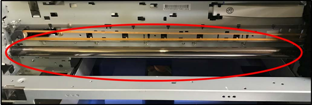
This is the Print Carriage Bar, the large chrome bar in the printer that the printhead uses to move left and right.
