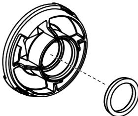
\*\* It is important that the nozzle seal inside the nozzle be re-installed properly. Make sure the cup side of the seal (the side with the groove) is facing out towards the front of the nozzle. Improper installation will cause leakage and damage to the turbine.
