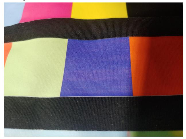
You'll notice this banding type effect mostly if the image has lower ink volume in certain areas. This can be confirmed by switching ink channels in Rip settings and if it does it with the other channels. If the nozzle check is at 100% you can try a higher resolution, the weave overlap function or turning up the color strength
