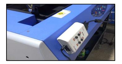
5. Place the Controller on the right side of the printer (magnets will hold it in place) and connect both the VGA and power supplycables into the controller.
