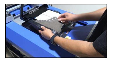
3. Mount the shoe onto the platen and press the fabric down onto the double-sided carpet tape to flatten the print area as much as possible.
