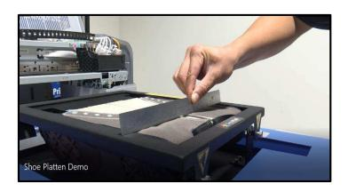
6. Using a ruler make sure that the shoes are evenly placed and flat with the top frame and look for any un-even surface to avoid a printhead head-strike.
