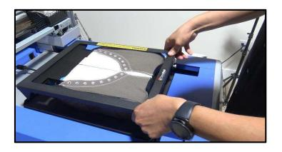
5. Repeat steps 4 and 5 to install the other shoe on the platen and close the top frame pressing firmly from both sides at the same time until the pins lock them selfs into place. Note: To lock the pins in place you might need heavy pressure but it's important to flatten the shoes properly.
