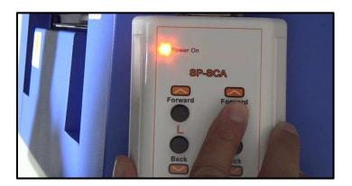
7. Test the platen mechanism by pressing each button on the controller and make sure that all of them are properly moving and operating as expected.
