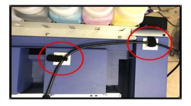
4. Secure the VGA cable onto the cable tie mounts using the hook and loop cables ties
