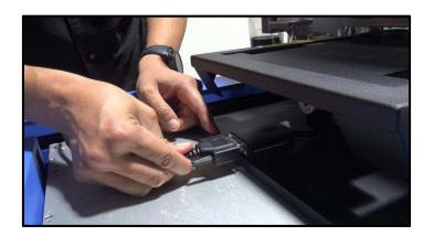
3. Connect the VGA cable into the back of the platen
