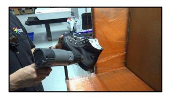
3. For best results, dry the pretreatment using a heat gun. If no heat gun is available, you may dry by hovering with a heat press but DO NOT PRESS.
