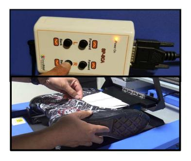
5. To release the shoe, press and hold the back button on the controller and remove the shoe carefully to avoid damaging the final print.
