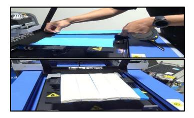
2. Place double-sided carpet tape onto the painter's tape where the shoe will be mounted. This will help to keep the shoe flat and in place
