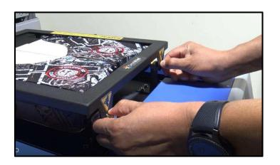
4. To release the top frame pull both pins and move the top frame upwards.
