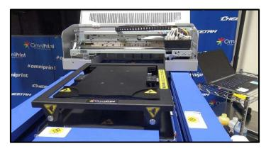
2. Place the platen on the printer with the pins facing the front
