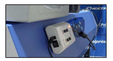
6. Switch the Controller ON and make sure that the orange LED light at the front of the controller is lit.
